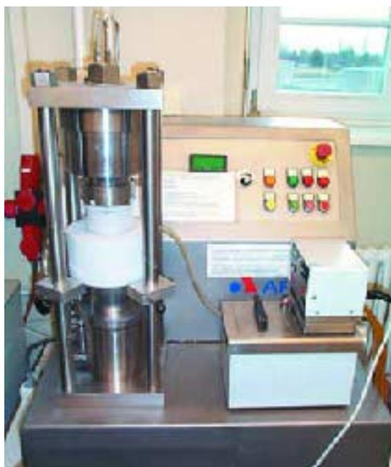
**3** Micron Lab 40, the homogenisation tower (front left) is equipped with a temperature control jacket (middle of tower) controlling the actual homogenisation chamber. There is an ice layer formed on the temperature control jacket by condensation from air humidity.
