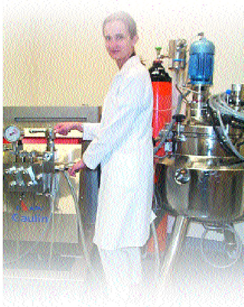
4 APV high pressure homogeniser (left) with a production capacity of 150 kg dispersion per hour, a product container for medium scale (right),
