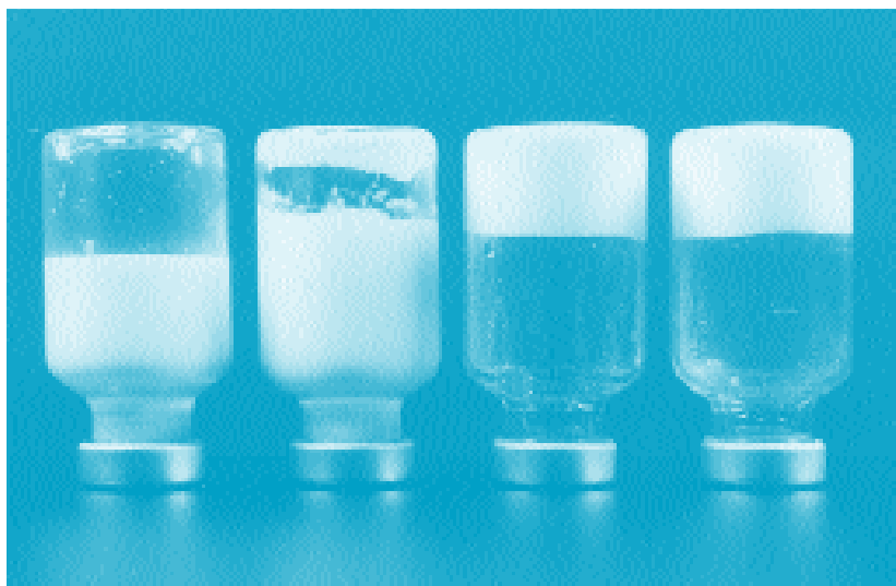
3 Appearance of lipid particle dispersions with increasing concentration of 20% and 30% (SLN, from left), more viscous NLC structure at 35% and high-viscous NLC dispersion (right) [after12].
